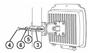
2. Fasten two M8×80 screws ④ and washers ⑤ through the drill holes and main bracket with a spanner;
